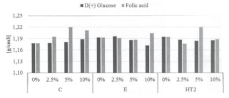
Fig. 3. Specific weight of epoxy resins with Glucose and Folic Acid
