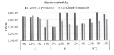
Fig. 4. Electric conductivity of NMP and DMF modified epoxy resins
