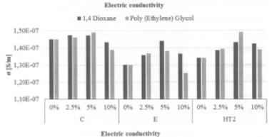
Fig. 5. Electric conductivity of Dioxan and PEG modified epoxy resins
