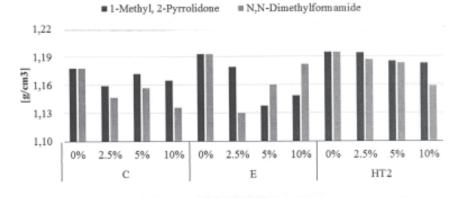
Fig. 1. Specific weight of epoxy resins with NMP and DMF
