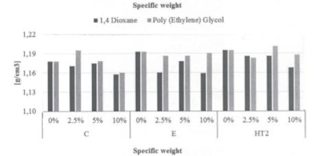
Fig. 2. Specific weight of epoxy resins with Dioxan and PEG
