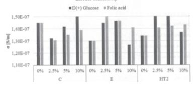
Fig. 6. Electric conductivity of Glucose and Folic Acid modified epoxy resins
